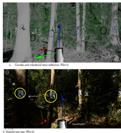
Figure 8. Illustration of circular and cylindrical retro-reflectors (a) and mounted tree tags (b).
