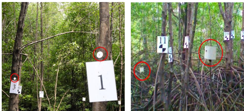
Figure 5. Both circular and cylindrical retroreflectors that used as a reference (the common point between the two-scanning position) to register the four-scanning position in sample plot. Circular (left) and cylindrical (right) retroreflectors used.
